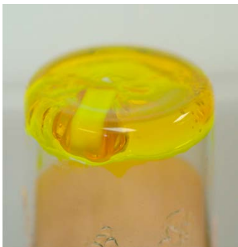
Figure 4. Photograph of a PFT hydrogel suspended in a vial upside down, trapping a magnetic stir bar and showing the resistance to viscous flow by gravity.
